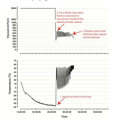
Secondly, once fully deep frozen, the vacuum pump removes the air from the camber. When the pressure in the camber reaches 0.066 kPa (500 mTorr), the trays are then gently heated (typically to around a maximum of 52°C).
