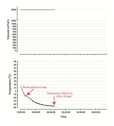
Firstly, the pepperberries are placed onto trays, a single layer thick, and then deep frozen to between -40°C and -50°C.
